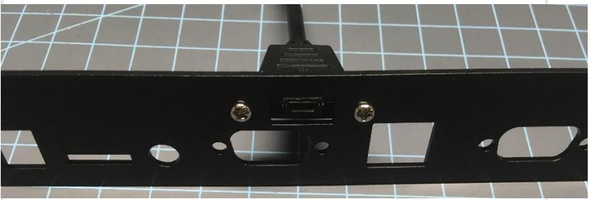
Remove the jack screws from the VGA and Serial connectors with a needle-nose pliers, or a 3/16" or 5mm socket.
