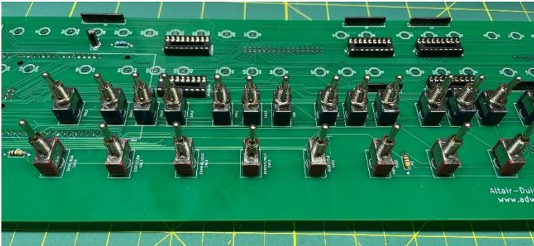
Be careful that you don't over-heat the toggle switches while soldering. This can damage the switch mechanism. Instead of soldering all three lugs on the toggle one after the other, I solder the top lugs on all switches, then the center lugs, then the bottom lugs like this:
