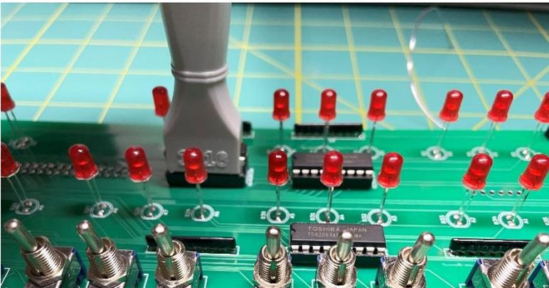
At this point you can put the Arduino Due in place.
