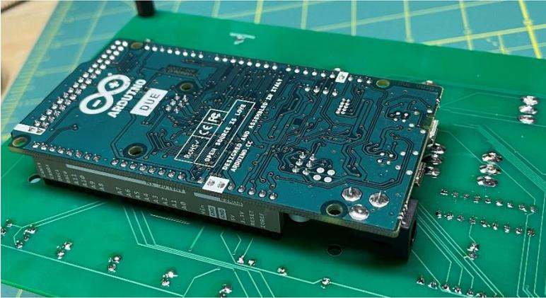
This is a good time to test your Altair-Duino. Plug a micro USB cable into your Arduino and connect it to a computer (or other USB power supply.) Try launching Kill-the-Bit by setting SW1 up and raise AUX1 as seen in this video: [adwaterandstir.com/FirstTest](http://adwaterandstir.com/FirstTest). Next, set SW0 through SW15 up and lower EXAMINE and see if all address LEDs illuminate. If not, check your solder connections.
