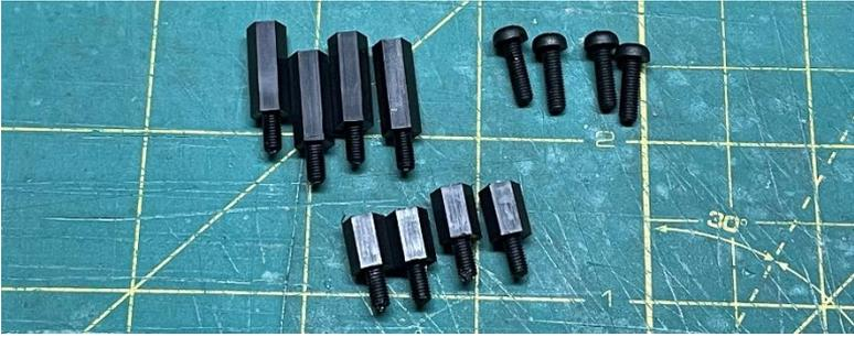
We're going to temporarily add the standoffs to the main circuit board with the 15mm on top and 8mm on the bottom.
