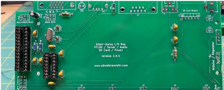
Cut two six-pin male headers and solder those to the upper left of the circuit board. Also add the 34-pin double header to the left side.
