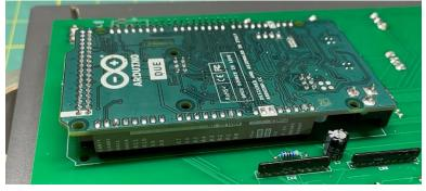
This is a good time to test your Altair-Duino. Plug a micro USB cable into your Arduino and connect it to a computer (or other USB power supply.) Try launching Kill-the-Bit by setting SW1 up and lower AUX1 as seen in this video: adwaterandstir.com/FirstTest.
