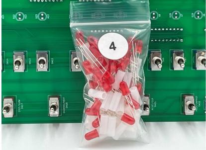
Place the main circuit board, top side up, on supports (like you did with the front panel earlier). Add 36 LEDs each with a 12mm standoff, paying attention to the correct polarity (long leg toward the top).
