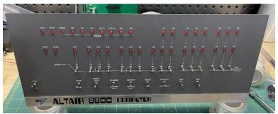
The front panel is complete. You can set it to the side as we work on the expansion circuit board.
