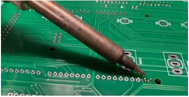
After all header pins have been soldered, remove the Arduino and place it aside for later.
