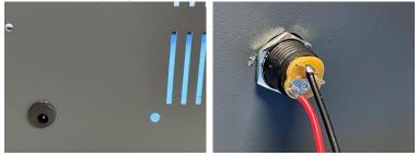
Would you rather power your kit with 110/220 volts? You can do this with the included strain relief bushing, a power cord, and a Mean Well RS-15-12 power supply (holes are cut in the rear of the case to match the mounting holes for this power supply). But this is optional and offers no enhanced performance or capabilities.
