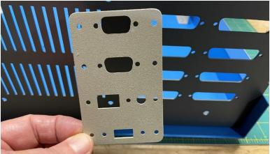
Take seven M3 bolts and seven M3 nuts from bag 6 and attach the ports panel as shown:
