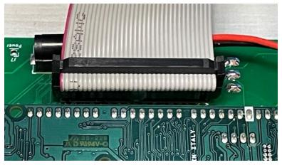
Plug the other end of the cable into the expansion circuit board. Again, note the orientation.
