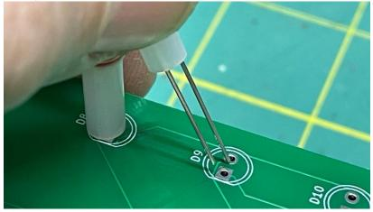
I like to support the circuit board at both ends and one support in the middle.
