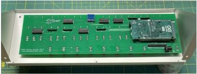
Hold the front panel in place and secure it with several toggle switch lock washers and nuts (that you previously removed from the switches). You can use an 8mm socket driver for this.
