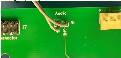
Solder the XH connector (should be plugged into the end of the incoming power cable) to the expansion circuit board exactly as shown (in this exact orientation):
