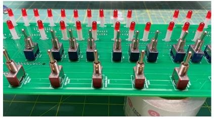
When all 36 LEDs and in place, put the front panel in place and flip the board over, placing it on your supports.
