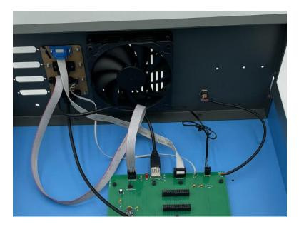
You can easily and inexpensively add one. Just look for a 120mm fan with 3-pin connector. They are available everywhere – Amazon, eBay, DigiKey, Mouser, Ali Express, etc. The fan will come with screws to attach it to the back panel, then just plug it into the expansion board connector.
