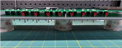
Be careful that you don't over-heat the toggle switches while soldering. This can damage the switch mechanism. Instead of soldering all three lugs on the toggle one after the other, I solder the top lugs on all switches, then the center lugs, then the bottom lugs like this:
